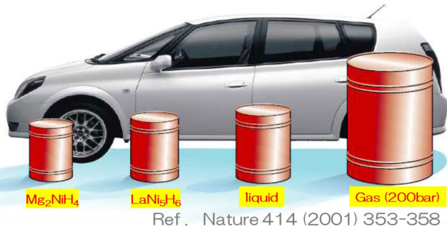
Figure 1 Volume of 4 kg of hydrogen compacted in different ways, with size relative to the size of a car. (Image of car courtesy of Toyota press information, 33rd Tokyo Motor Show, 1999.)
